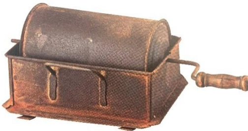
Image 2: Coffee roasting tool with a cylindrical chamber that rotates around a shaft and roasts the coffee in a covered housing, Nihal-Murat Sungur Collection, Bursa
